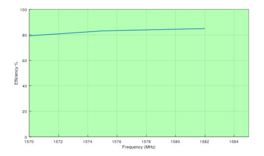
\*Data are given for antenna on 70x70 mm metal ground plane.
